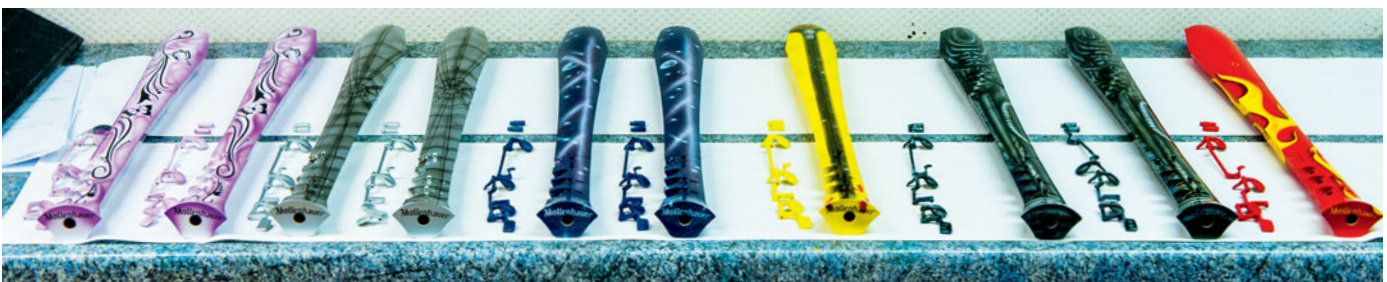
The so-called 0-series of Elody in their different finishes: the externally finished instruments require the mounting of the key mechanism as well as the drilling of finger-holes and cutting of windway and labium.
