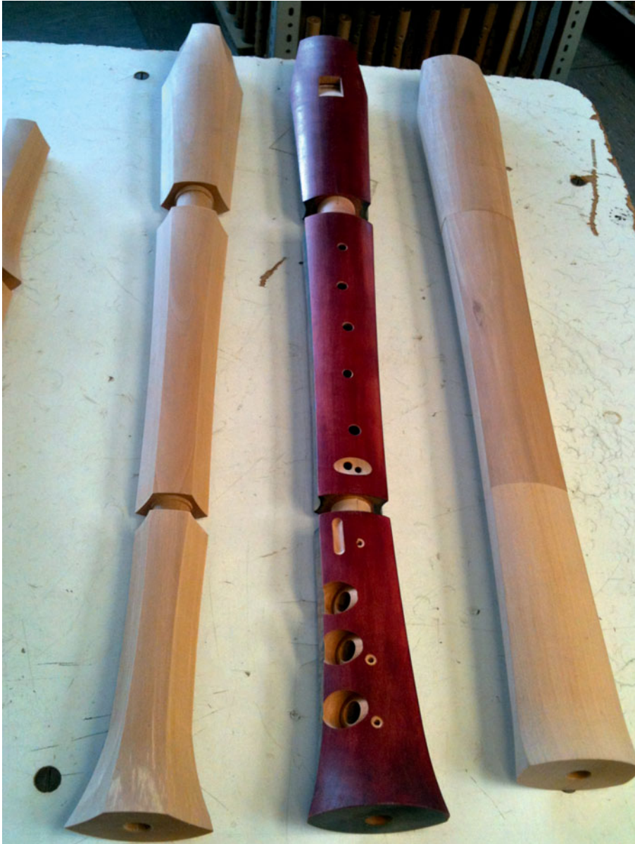
Different shapes of Elody prototypes in their crude stage – stained in trial colours.
