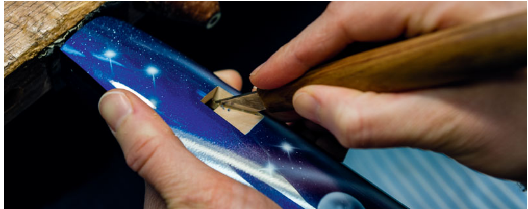
Various stages of the production of the Elody at Mollenhauer: fixed in a vice for the drilling of the middle part, the mounting of the keys and the re-cutting of the labium.
