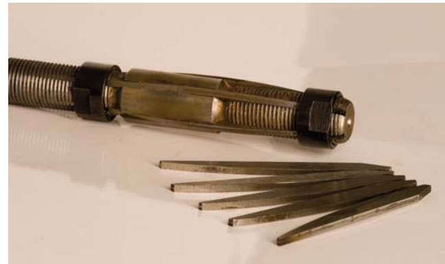
Adjustable six-bladed reamer for making prototypes or experimenting with bores
